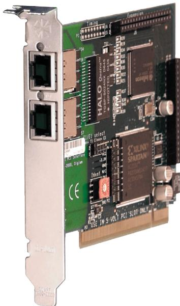
The TE205P and TE210P support industry standard telephony and data protocols, including Primary Rate ISDN (both N. American and Standard Euro) protocol families for voice, PPP, Cisco, HDLC, and Frame Relay data modes. Both line-side and trunk-side interfaces are supported, also included are advanced call features.
